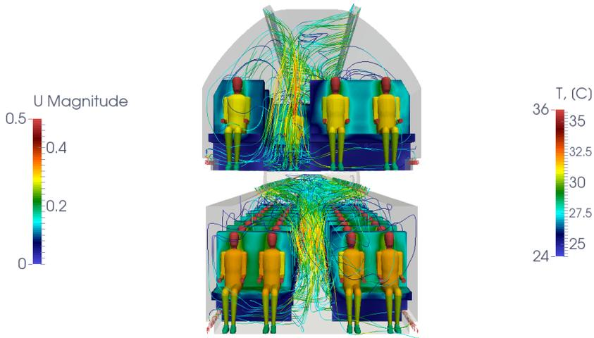
**Fig. 2** Streamlines emerging from inlet surfaces colored with the velocity magnitude and temperature distribution on passenger bodies.
