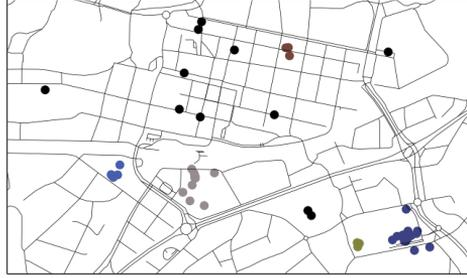
**Fig. 2** DBSCAN  $\epsilon = 200$  m. Points with similar color are categorized into one cluster where noise points are depicted in black. By increasing the  $\epsilon$  value from 100 to 200, compared to Fig. 1, the points in the parking lot are clustered together, while many of the noise points (corresponding to distinct destination) in the city center are merged into one large cluster.
