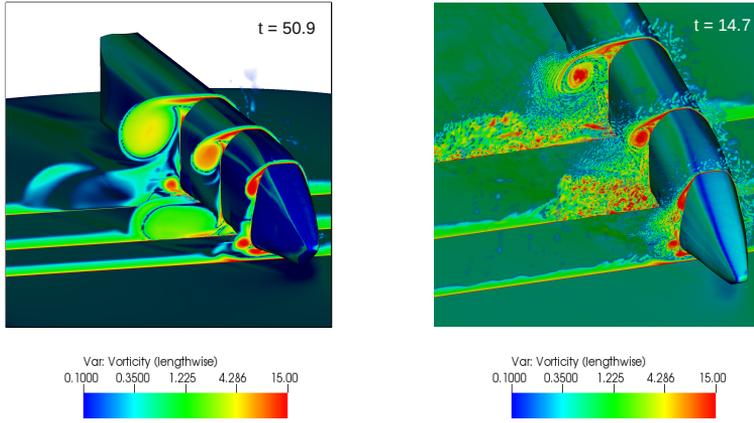
**Fig. 1** Instantaneous vorticity (in train length direction) for three different slices of the incompressible URANS (left) and DDES (right) simulation. Also shown is the stream-wise component of wall shear stress on the train surface. Time is expressed in units of convective timescales.
